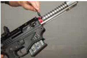
Photo 12-) Use your TR-12 Special Wrench Set turning the barrel nut of your gun.
