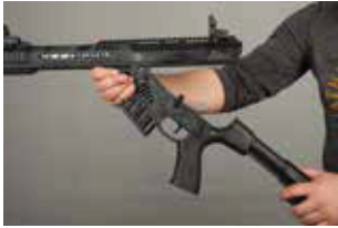
Photo 8-) You will be able to separate upper and lower frame of your gun after these steps as in the photo starting to disassemble forend of your shotgun, easily in right way.
