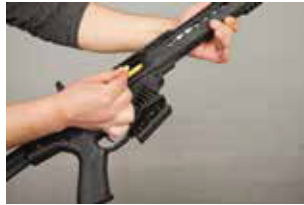
Photo 2-) Pull TR 12 charging handle to operation direction then use shell safety kit (yellow part) to make ready your gun disassembling in right way. If you do not use that shell safety kit, you will damage shell carrier ramp absolutely!!!
