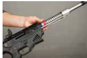
Photo 13-) You can disassemble bolt group of TR-12 completely after required steps as in the photo easily.
