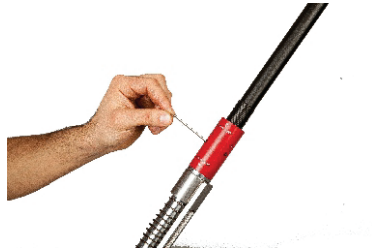
Photo 11-) Unscrew the fixing screws which are on the gas cylinder with 2,5mm allen wrench
